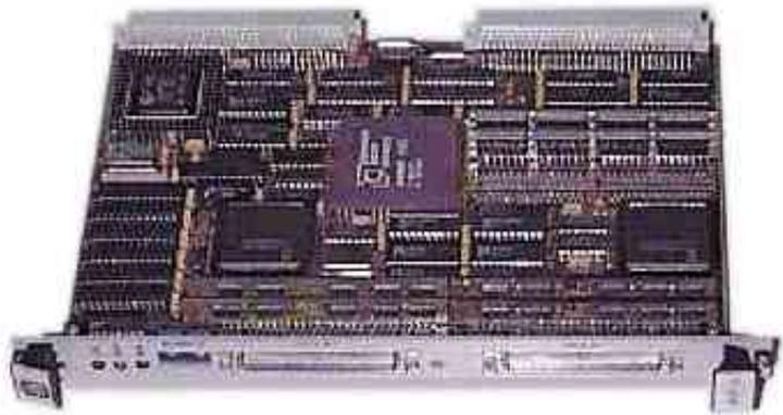
The Macrolink MVC 16-port Communications Multiplexer is the first VMEbus Async Commux designed for real performance. Unlike traditional controllers that rely heavily on the host for processing or 68XXX-based controllers that still can't meet high through-put requirements, the MVC has processing power to spare thanks to the AMD 29K. The MVC provides outstanding flexibility and one of the most comprehensive set of features available today-all at a very affordable price.
